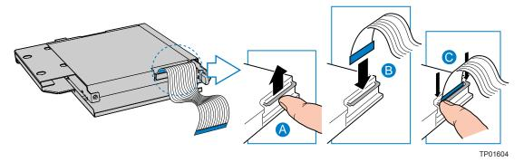
Figure 21. Installing Floppy Flat Flex Cable to a Floppy Drive
